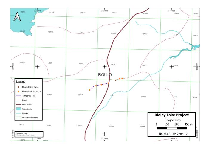
In total, there are 6 drill pads planned in the Rollo township to prove the eastern extension of the veins. The location of the planned drill holes is favorable for penetrating the known veins identified in previous drill campaigns. Geophysics indicates the extension of the structural trend to the east; therefore, this area can host additional gold-bearing veins.
