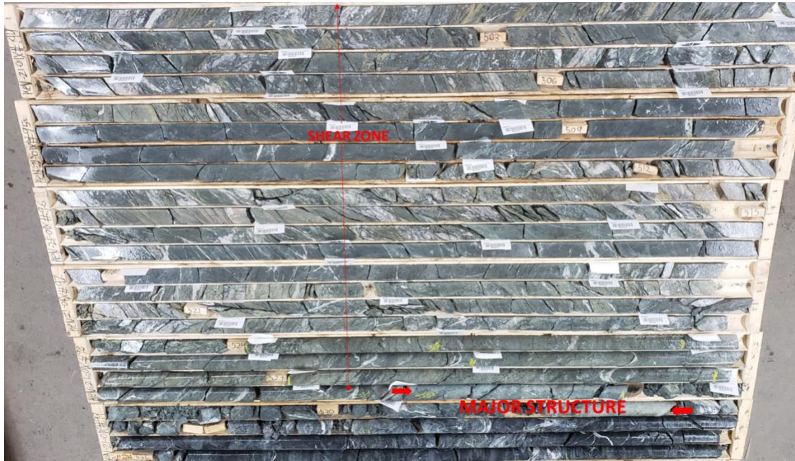
Figure 2 Major Structure Core
