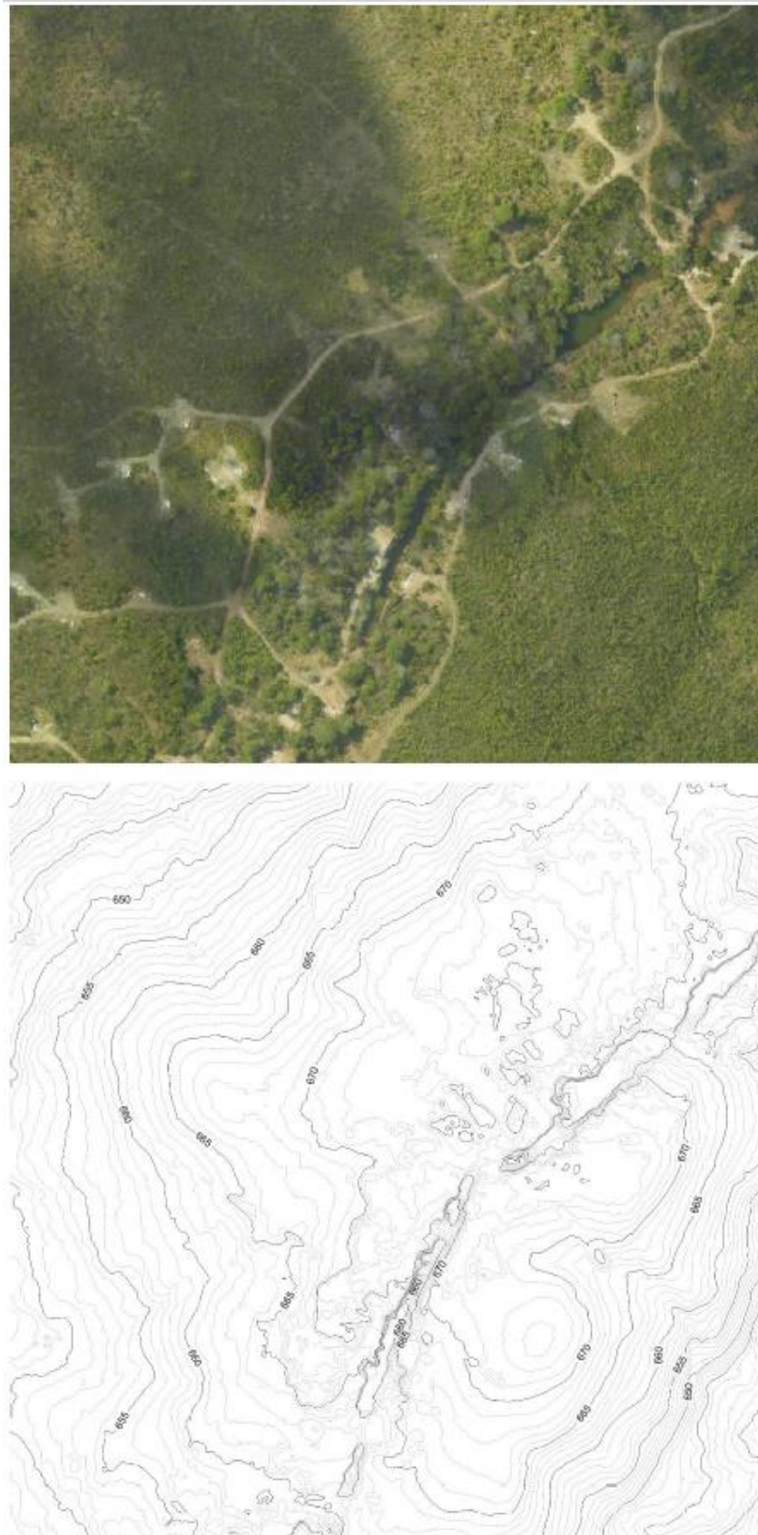
Figure 14-3 An example of the LIDAR topography's ability to identify surface depressions of garimpos.
