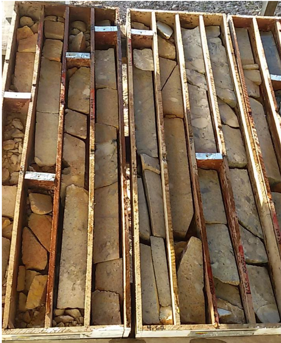
Figure 16-4 Drillcore boxes in the shallow saprolitic zone with two fracturing families
