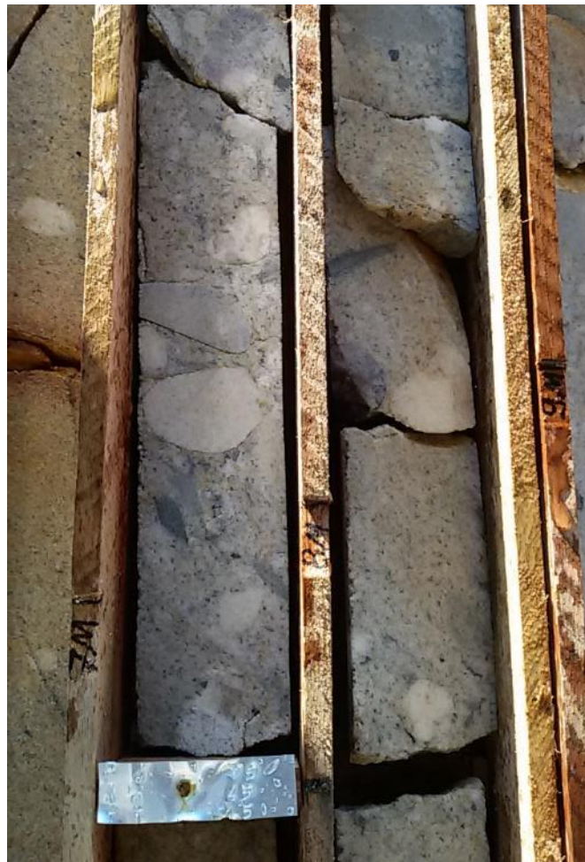
Figure 16-6 Drillcore box in fresh rock zone showing conglomerate intercept
