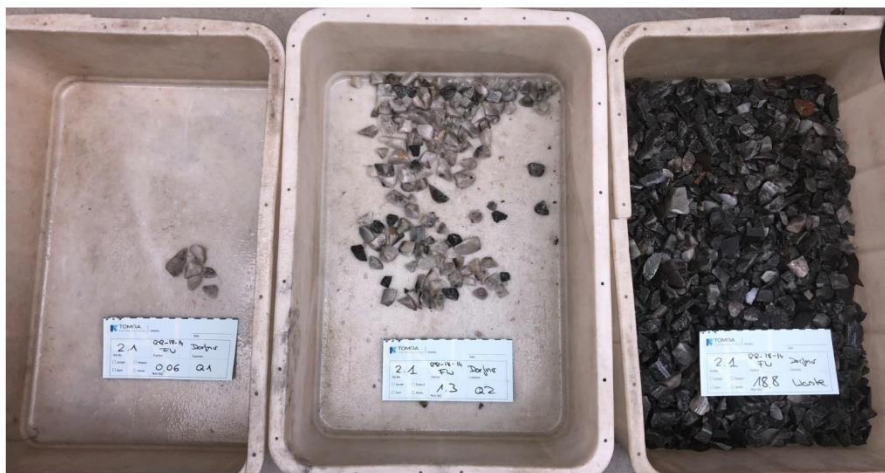
Figure 9: Fractions Q1, Q2 and waste after two step optical sorting of sample FW from drill core RR-18-14
