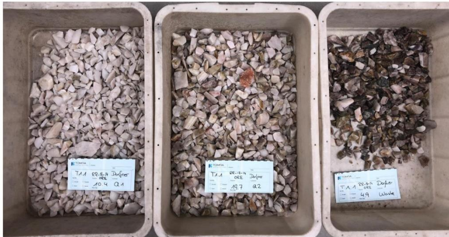
Figure 8: Fractions Q1, Q2 and waste after two step optical sorting of sample ORE from drill core RR-18-14
