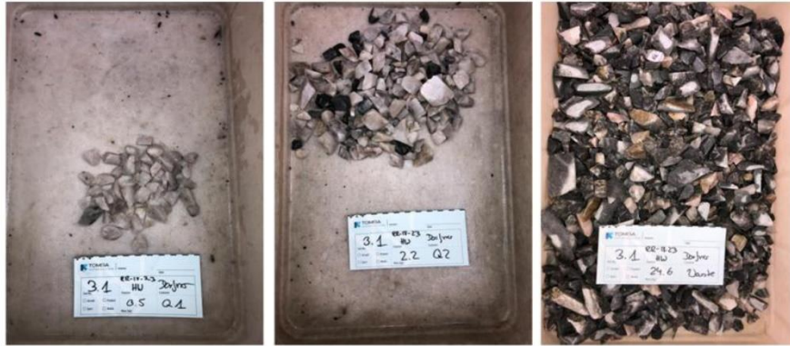
Figure 10: Fractions Q1, Q2 and waste after two step optical sorting of sample HW from drill core RR-18-23
