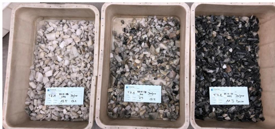
Figure 14: Fractions Q1, Q2 and waste after two step optical sorting of sample ORE from drill core RR-18-28
