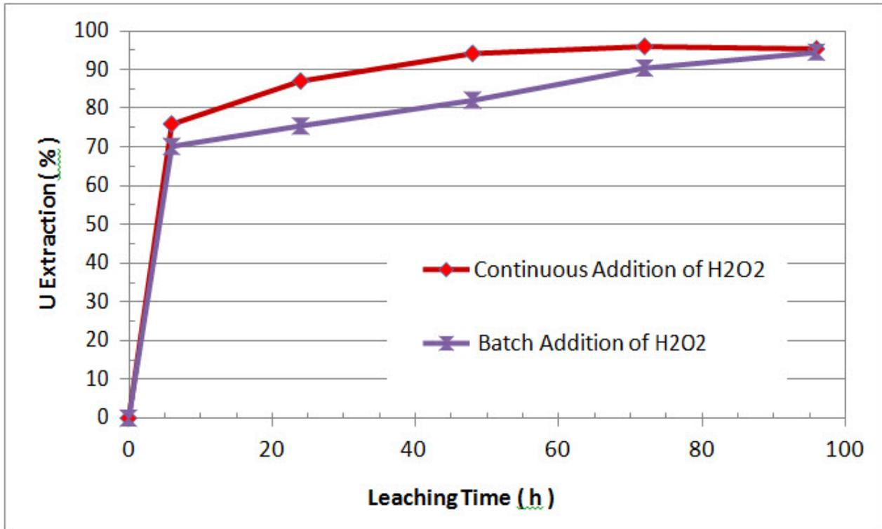
Figure 13.7: Leaching kinetics with different oxidation
