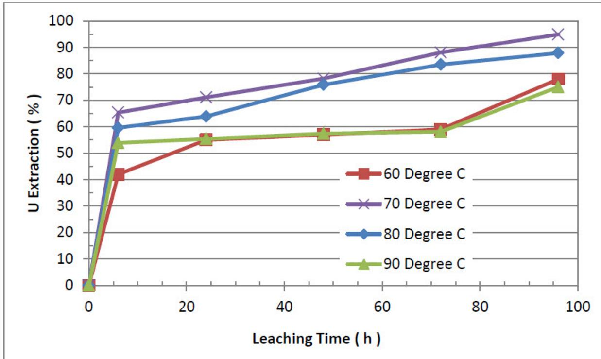
**Figure 13.5:** Whole ore U alkaline leach at variable temperatures
