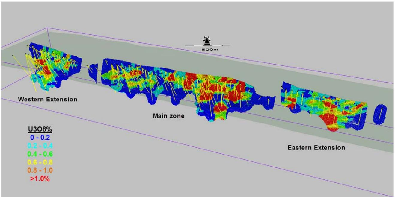
**Figure 14.18:** Distribution of Inferred Resource Above 0.2% U<sub>3</sub>O<sub>8</sub> Cut-off – J4 / Ray
