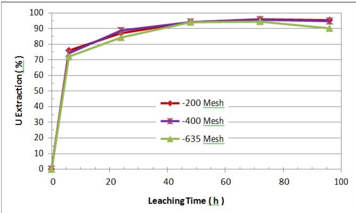
Figure 13.8: Leaching Kinetics of Different Size Feeds.
