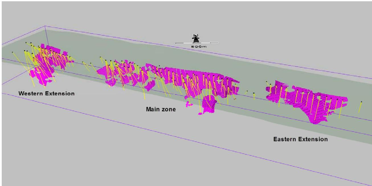
**Figure 14.16:** Distribution of Inferred Resource Above 0.2% U<sub>3</sub>O<sub>8</sub> Cut-off – Lac Cinquante
