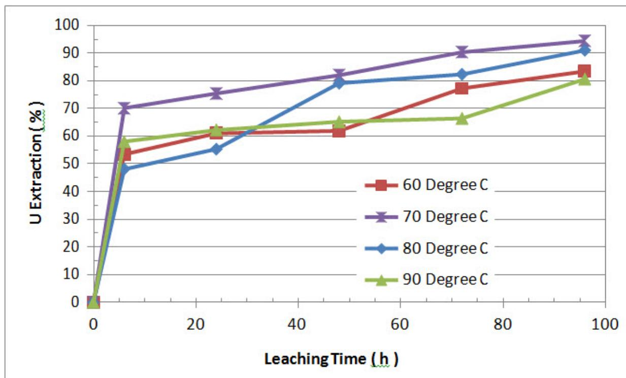
Figure 13.6: Flotation tails U alkaline leach at variable temperatures
