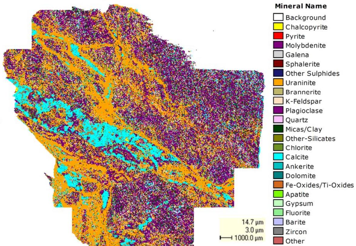
**Figure 13.1:** QEMSCAN™ Pseudo Image of Sample 90001 illustrates structural control of U mineralization among silicates and carbonates
