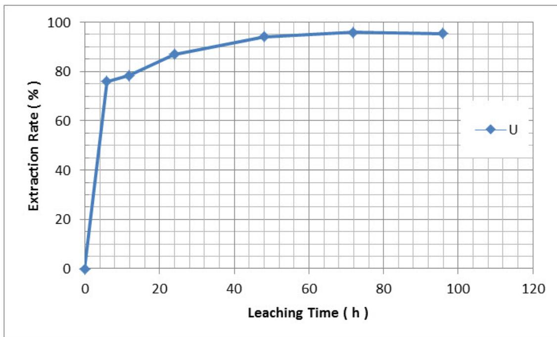
**Figure 13.4:** Optimized alkaline leaching kinetics of uranium
