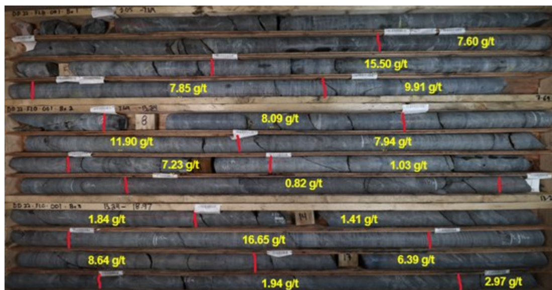
Figure 1: DD22-FLO-001 core photo of the majority of the 17.4 m of 6.52 g/t Au interval; grades listed on core.
