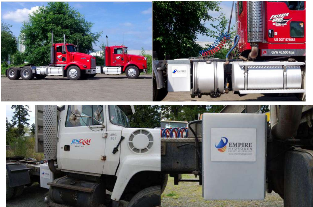
Jencam and Freisen Bros. Trucks used in ABPTDP – Displaying Mounted A/Gs
