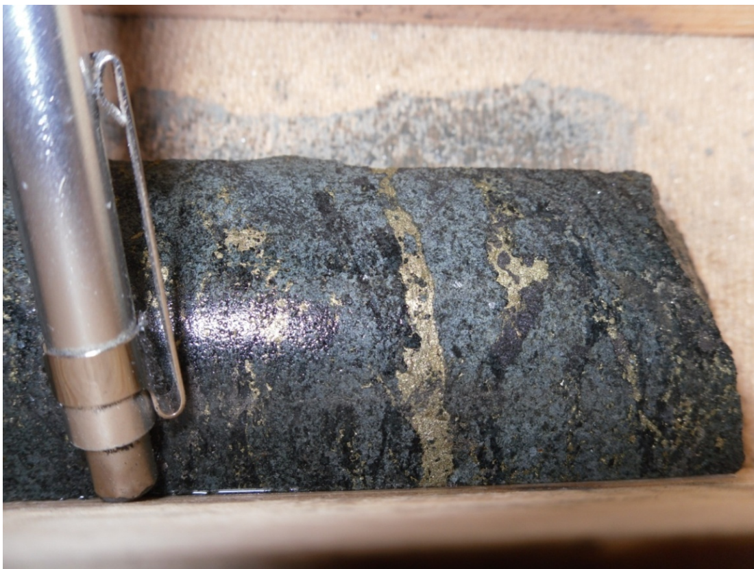
Figure 6-5: Drill core showing veins of magnetite and chalcopyrite/pyrite in skarn (Source: SRK February 2011)
