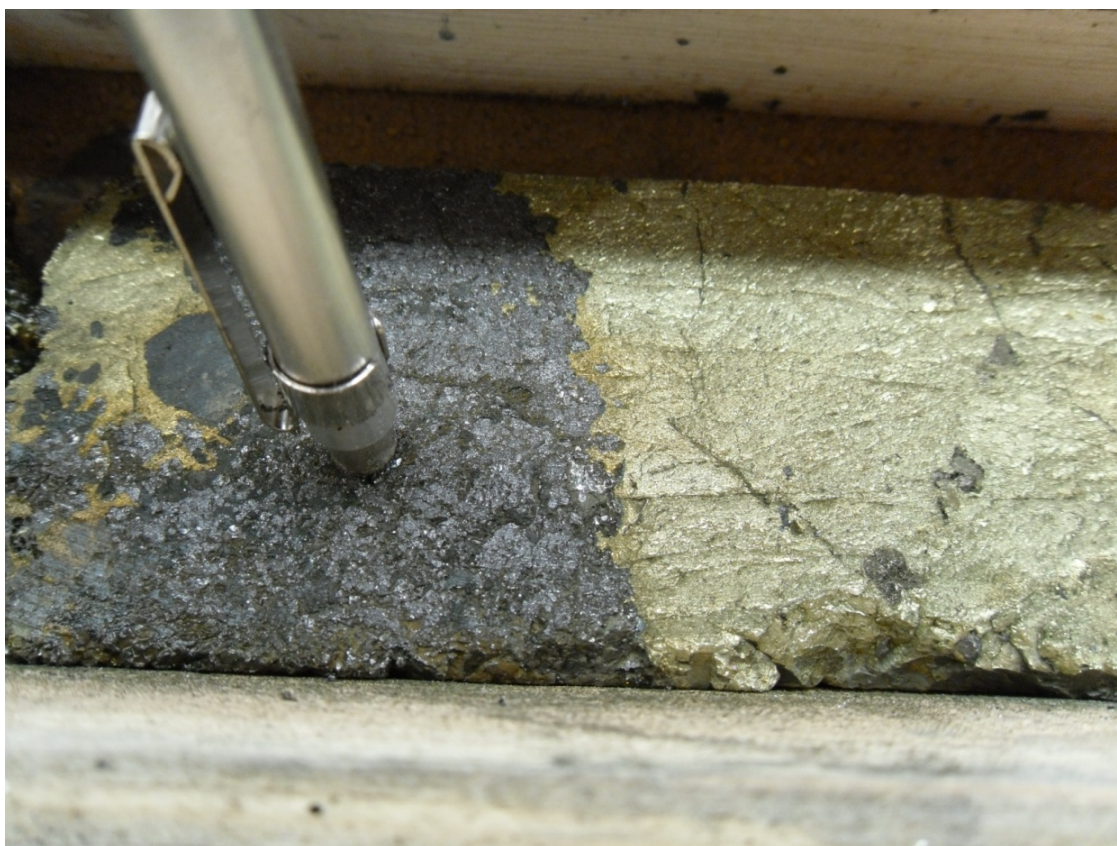
Figure 6-4: Drill core showing massive magnetite and chalcopyrite (Source: SRK February 2011)
