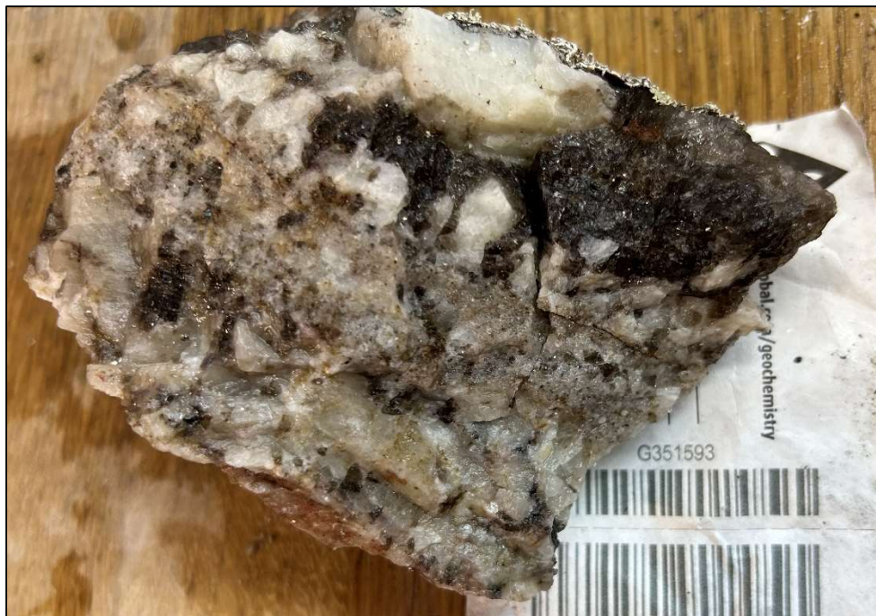
Fig 1: picture of sample G351593 (88ppm Li) showing a zoned crystallization with layers of K feldspar, quartz (dark brown) and fine grain muscovite.
