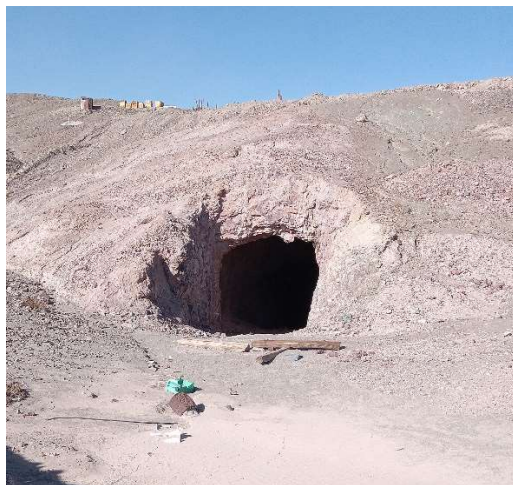
Figure 2: shows the decline entrance on the La Fortuna mine from which up to 14% copper material was historically mined.
