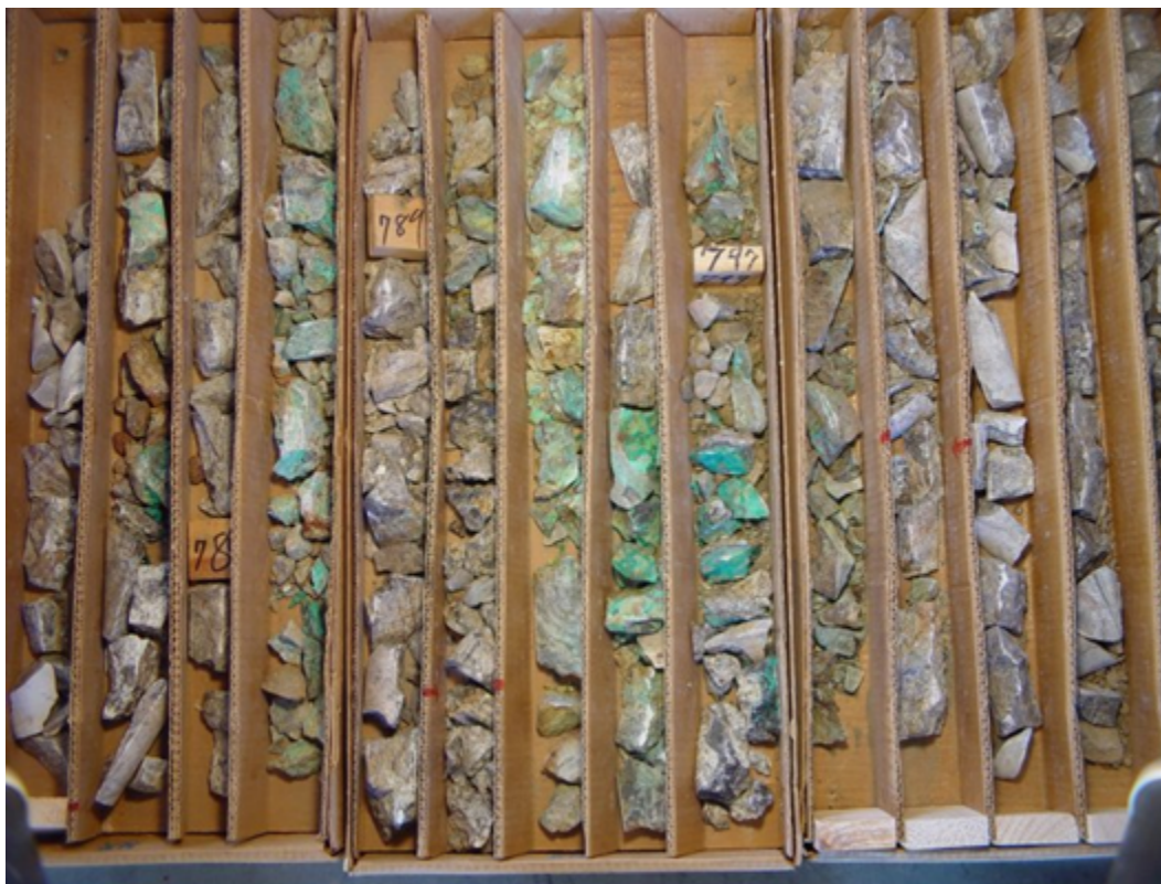
Figure 7-8: Photograph of Typical Oxide Mineralization for the Gunnison Deposit Hole J-9: 780 to 806 feet
