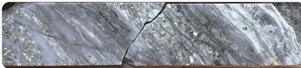
Figure 11: High volume sheeted veins of quartz (qz), chlorite (chl), pyrite (py), chalcopyrite (cpy) and carbonate (cb), Cliff porphyry (M-23-001, 165.5 m)
