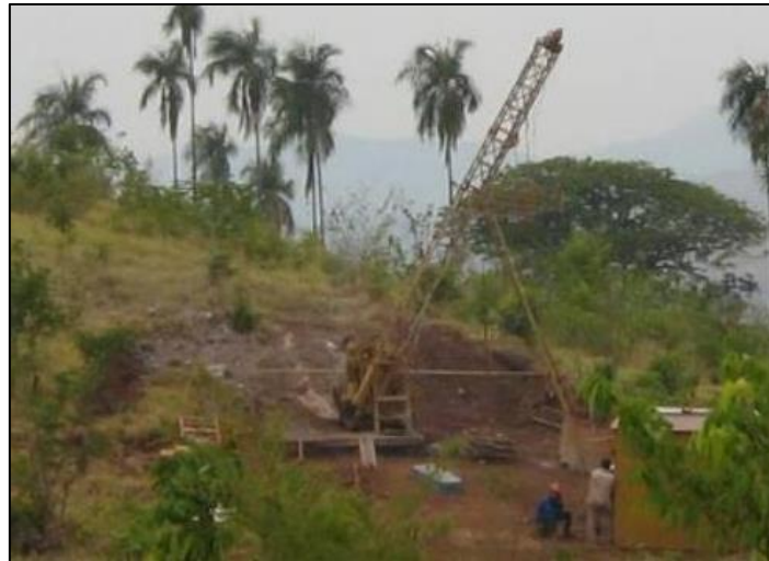
Figure 10-2: Drilling under DOCEGEO administration at Luanga Project, angled drill hole
