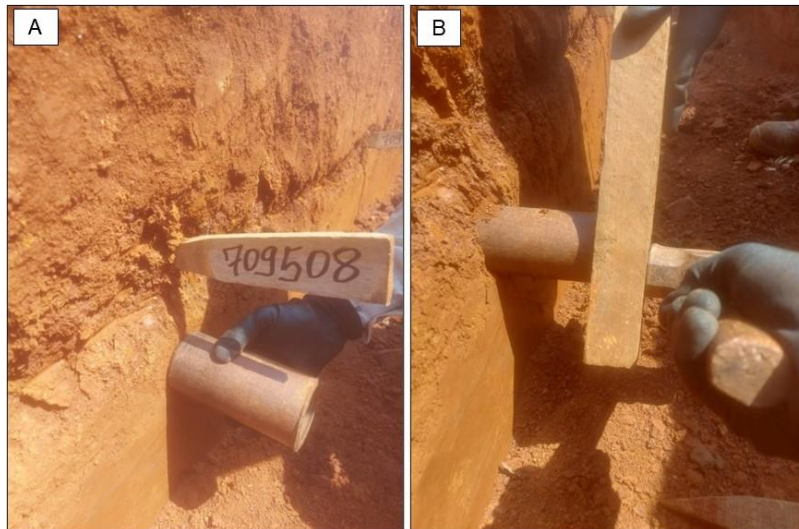
Figure 9-20: Cylinder insertion into weathered material
