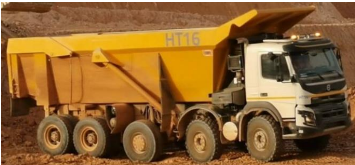
Figure 16.27 – Typical 10 x 6 Haul Truck
