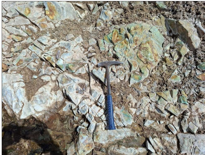
Figure 12-3: Intensely Brecciated Quartzite Infilled with Authigenic and Allochthonous Oxides
