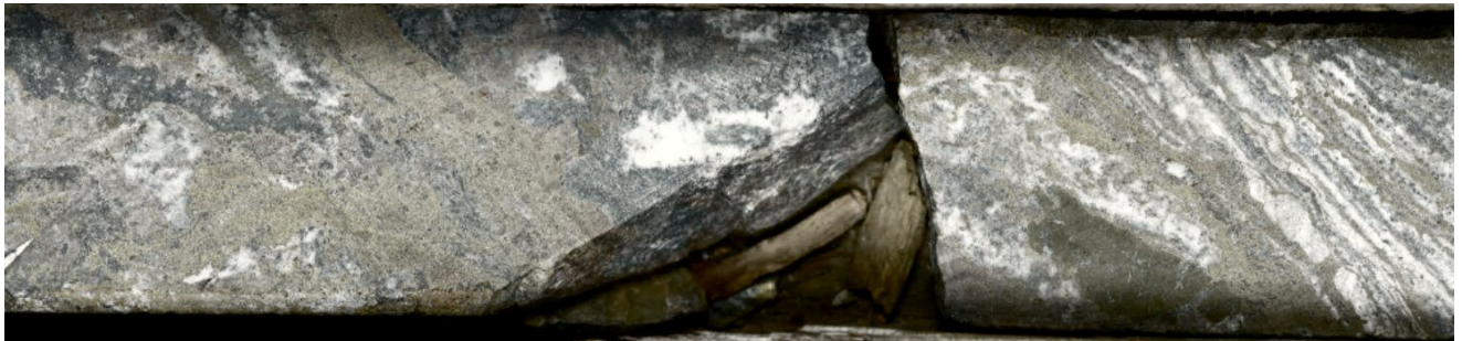
Figure 7-13: Quartz-Sulphide Facies from JS81-068W1
