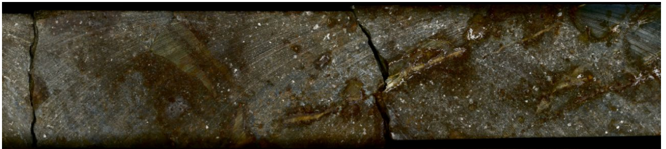
Figure 7-14: Massive Pyrite Facies from JS82-086W1
