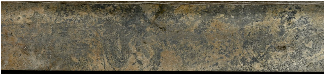
Figure 7-15: Ferroan Carbonate Facies from JS80-056W1
