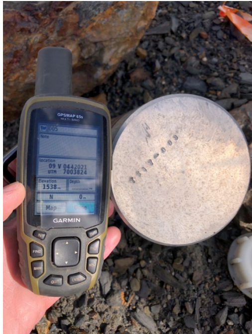
Figure 12-1: Collar Location Field Check (TS17-003)
